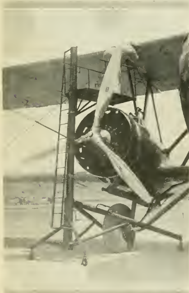
Portable servicing platform used by Eastern Air Lines at its servicing base
